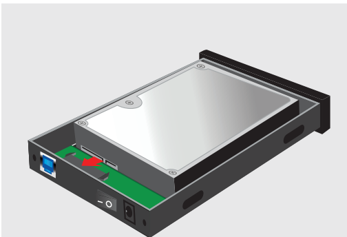
5. Push the drive in the direction shown to fully connect the SATA interface.
